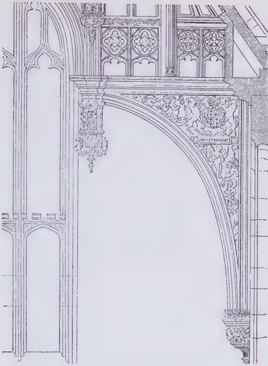
207 Hampton Court, great hall, hammerbeam roof, 1533
