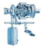
In the 6-99 there is an interesting innovation in transmission systems. Within a manually operated three-speed gearbox, with synchromesh or all three gears, an overdrive gear can, by the operation of a post-pull control, be brought into operation with either of the two upper gear ratios. This in effect provides five forward gears.
