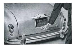
The lid of the luggage locker is counterbalanced for ease of opening. At night the lid handle is clearly illuminated by the number-plate light to facilitate unlocking.
