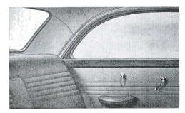
The rear corner roof panels are remarkably narrow because of the exceptional width of the curved rear window. This effectively reduces blind spots when reversing.
