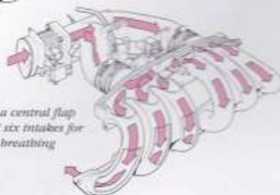
The 'Dual Ram' intake system means that the 2.6i engine and 3.0i 24-valve unit reach peak torque extraordinarily early. Up to 4000 rpm, the engine draws air through two separate groups of three pipes (shown left).
