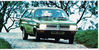
Engines: '1300': 1256cc OHV 4-cylinder. Bhp (DIN) 58,5@ 5600rpm. Torque (max) 68 lb/ft@ 2600rpm. Viscous drive fan. Mph per 1000rpm in top gear: 16-1.
