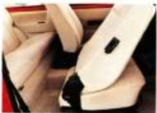
Special front seat tilt arrangement gives extra easy access to roomy rear compartment.
