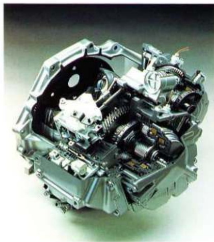
Cavalier's 4-speed automatic transmission is a highly sophisticated unit with three selectable driving modes.
