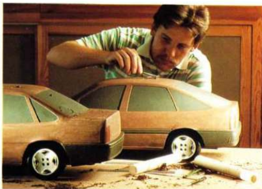
Scale models in clay – an early stage of the design process.
