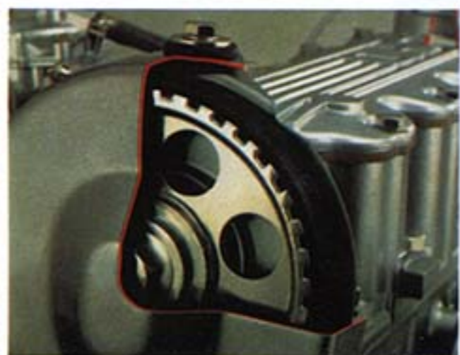
The overhead camshaft is driven by a hard-wearing toothed belt. It's silent, needs no lubrication and adjustment is easy.
