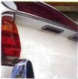
The Estate has the same 'full-flow' heater/ventilation system as the 2000. Ventilation ducts are located in the tailgate.
