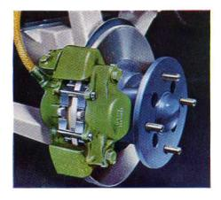
The Triumph's braking is as exceptional as its performance. Triumph enter the world's top rallies to test to the utmost. The result, bigengine performance is matched by bigengine braking. The Triumph 2000 has disc brakes at the front, where 70% of the braking effort is developed. Fast stops. No wet drums, no fading.
