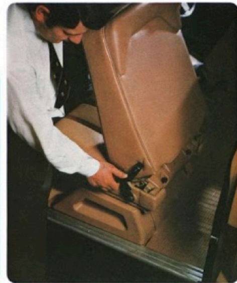
Right. Front seat backs can be released from outside or inside the vehicle and tipped forward, the movement automatically causing the whole seat to slide forward on its runners to facilitate access into the rear compartment.
