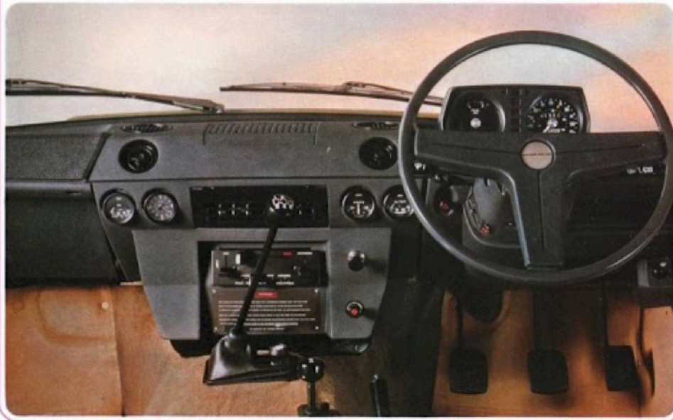
Main instruments and indicator lights are visible at a glance, and all controls are easily operated. The fascia is made of impact-absorbing material.
