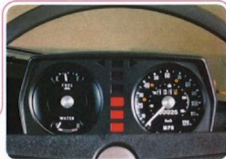
Main instruments and indicator lights are visible at a glance, and all controls are easily operated. The fascia is made of impact-absorbing material.
