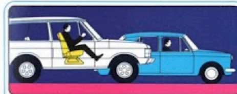
Right. Front seat backs can be released from outside or inside the vehicle and tipped forward, the movement automatically causing the whole seat to slide forward on its runners to facilitate access into the rear compartment.
