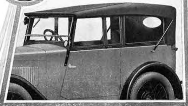
Showing the all-weather equipment in position.
