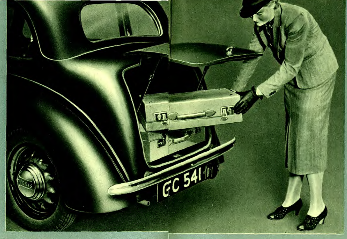
On the Saloon models the large inbuilt luggage container has external access by hinged lid with door-type lock. The capacity of the container is nearly 5 1/2 cubic feet.
