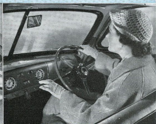
Gear change lever is on the steering column of the larger Morris models—to keep the driver's hand always near the steering wheel. Now it's easier than ever to change gear.
