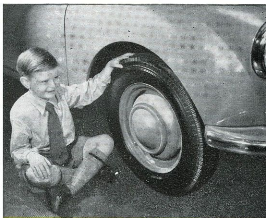
Low-pressure tyres increase riding comfort. Large section long-wearing tyres provide better road grip and a safer, surer "straight-line" stop in emergencies.
