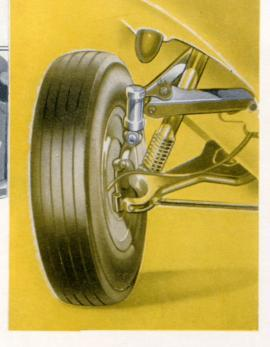
Long torsion barsin the independent front wheel suspension systemmake light of bumps and potholes. Side sway is eliminated by the semielliptic springing at the rear and the telescopic dampers all round.
