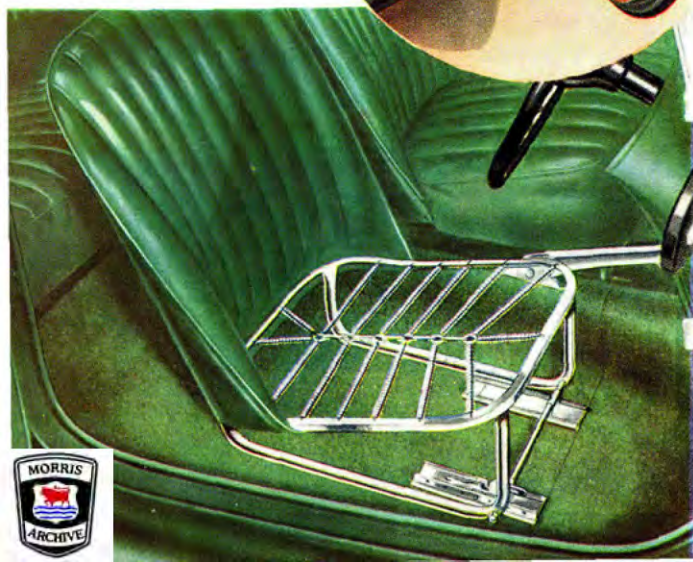
The front seats are of the metal framed easy-chair type with floating spring seat base.
