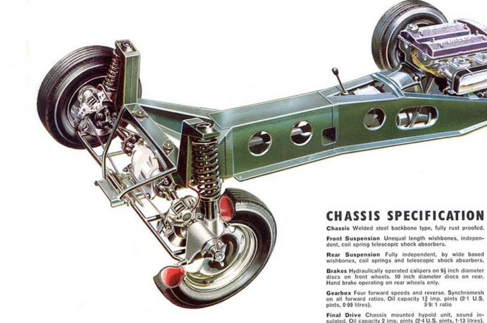
Steering Rack and pinion, with telescopic and collapsible steering column. Optional right or left hand drive, 15 inch diameter dished wood-rimmed steering wheel,  $2\frac{1}{2}$  turns
