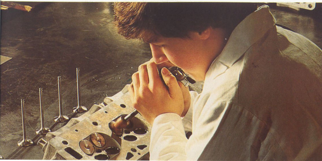
The hand lapping of cylinder head valves.
