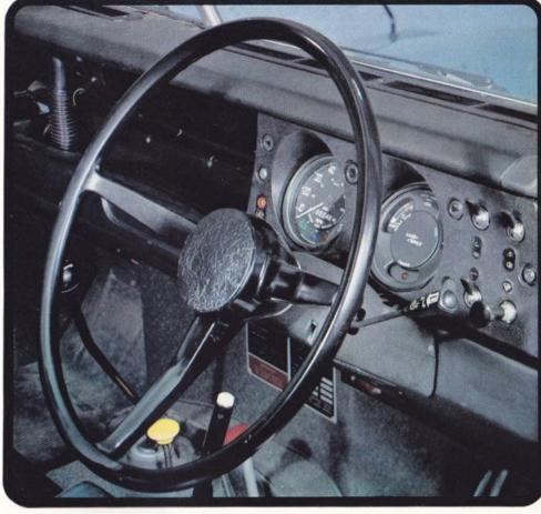
Driving a Land-Rover Station Wagon can be a very satisfying experience. The comparatively high seating position affords an excellent view of the road or ground ahead. Instruments are grouped in a binnacle within the driver's line of vision together with ancillary controls. Direction indicators, horn, headlamp flasher and dip switch are all operated by a single finger-tip control on the steering column.
