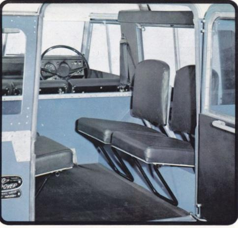
the vehicle. A folding mounting step is provided to assist entry.
