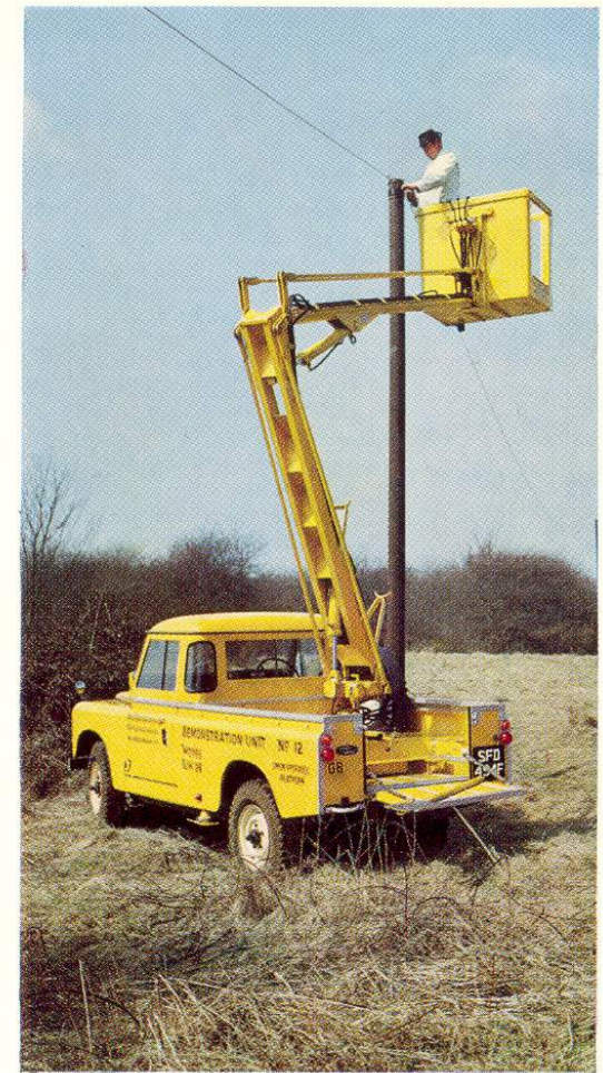
The vehicle provides an effective base on which to mount a hydraulically operated lift-platform. This type of equipment is in current use with many civic authorities for high-level maintenance tasks.
