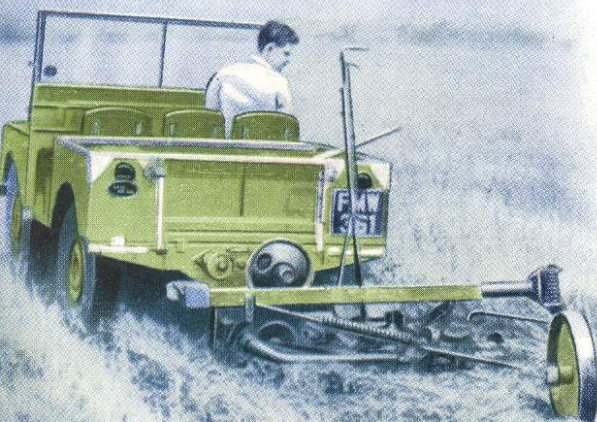
Operating a power-driven mower—one of the many uses of the rear power take-off.
