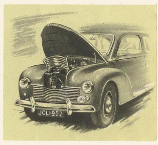
Outstanding engine accessibility that the ownerdriver has demanded for years; open the bonnet and the top half of the grille pivots up; the lower half of the grille is easily removable for major adjustments.
