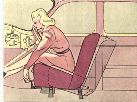
Correctly adjustable driving seat. Turn an easy handle below the seat and you raise and incline the squab; wind the seat forward or back to give safety and comfort for drivers of all heights, men and women.
