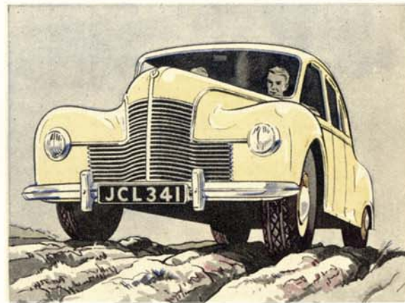
Ground clearance designed for rutted tracks, bad pot-holes and the worst surfaces that cars can travel. A minimum of 7 1/4 in. is just one of the many essential overseas features incorporated in the "world-market" JAVELIN.
