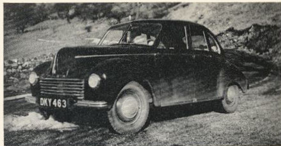
Much testing took place on Yorkshire test hills, including Sutton Bank. This is the second prototype with its designer at the wheel; it will be noted that the four doors are no longer interchangeable (as they had been on the first prototype) but all panels are very flat, for fabrication by simple methods. Bonnet and grille were changed before the car went into production, and at this stage a flat two-piece Vee windscreen was used.
