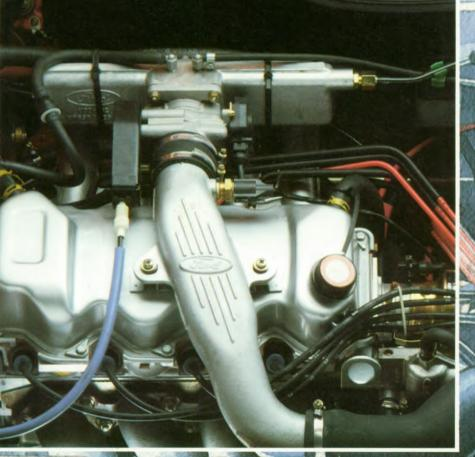
the turbo's 'wastegate', a high-tech safety valve which keeps boost pressures within the preset operating limits.
