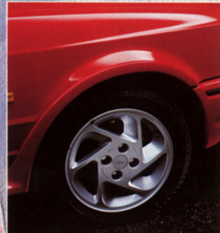
The light alloy 6x15 wheels fitted with 195/50 VR 15 tyres, providing large reserves of grip for sure-footed cornering and razor-sharp handling are standard on the Escort RS Turbo.
