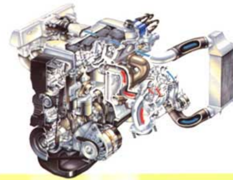
The turbo installation on the Escort RS features an air-to-air intercooler and revised inlet porting to increase power output.
