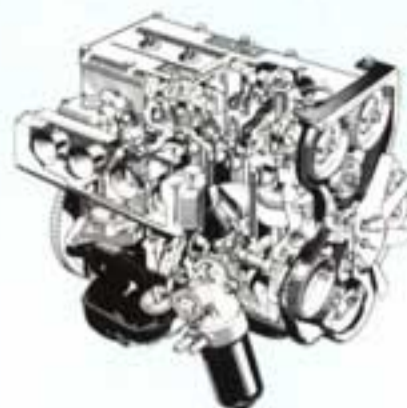
Cutaway drawing of the BDA engine, showing the 16-valve layout, and the belt drive to the camshafts.
