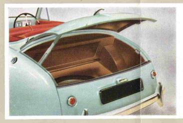
An enclosed and exceptionally roomy luggage compartment is located at the rear of the car. It accommodates the spare wheel and affords generous space for baggage of all shapes and sizes. The lid of this compartment, on being fully raised, is automatically held open by a supporting stay.
