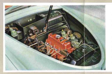
Compact in design, smooth and crisp in operation, the A40 Sports engine is a 4-cylinder o.h.v. unit employing twininclined S.U. carburetters and developing 50 b.h.p. at 4,800 r.p.m. That so much power is produced by so small an engine is a tribute to Austin designers and craftsmen.
