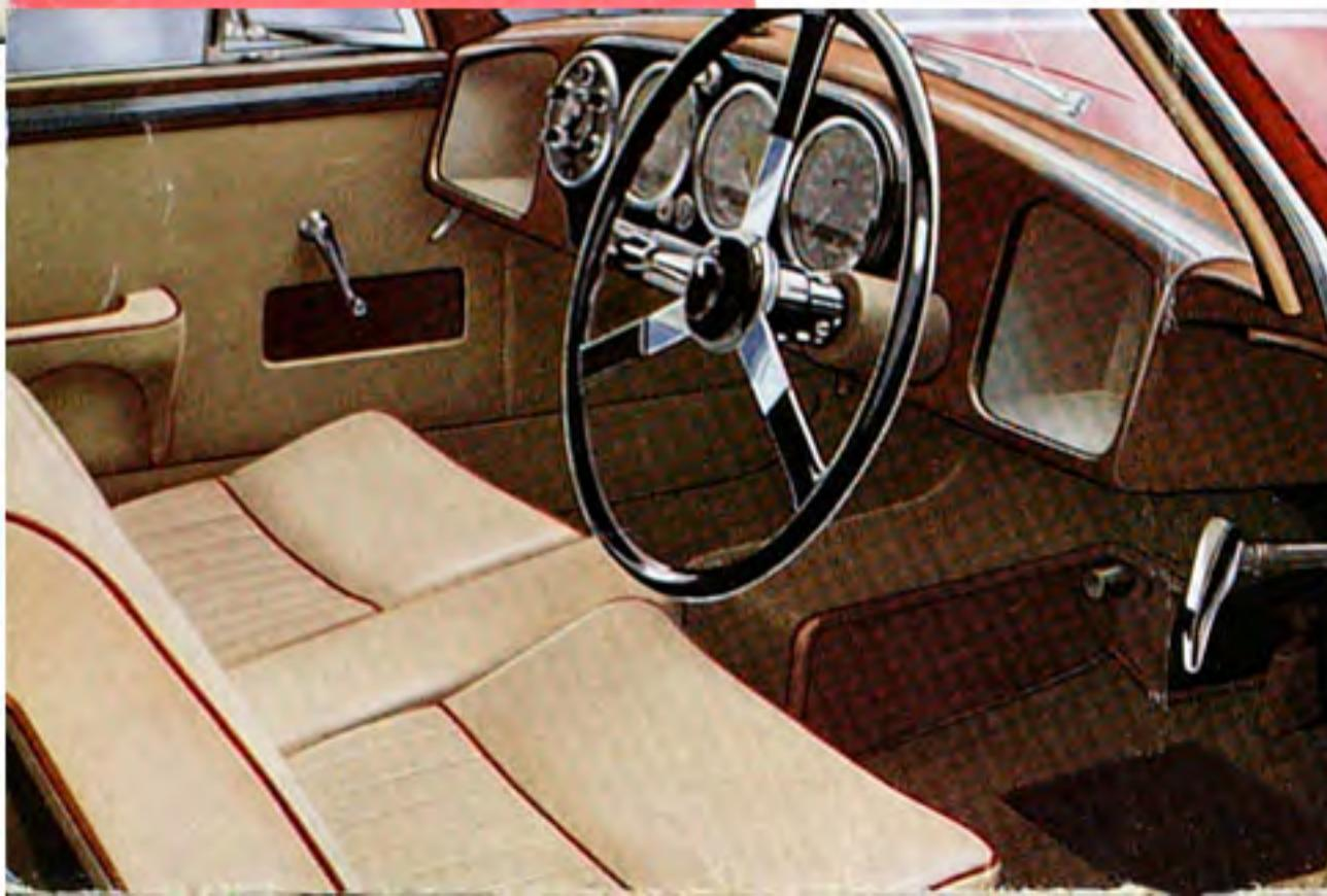
Full range of instruments includes speedometer, milometer and trip recorder, rev. counter, clock, petrol and oil capacity gauges, oil pressure gauge, coolant thermometer and ammeter.
