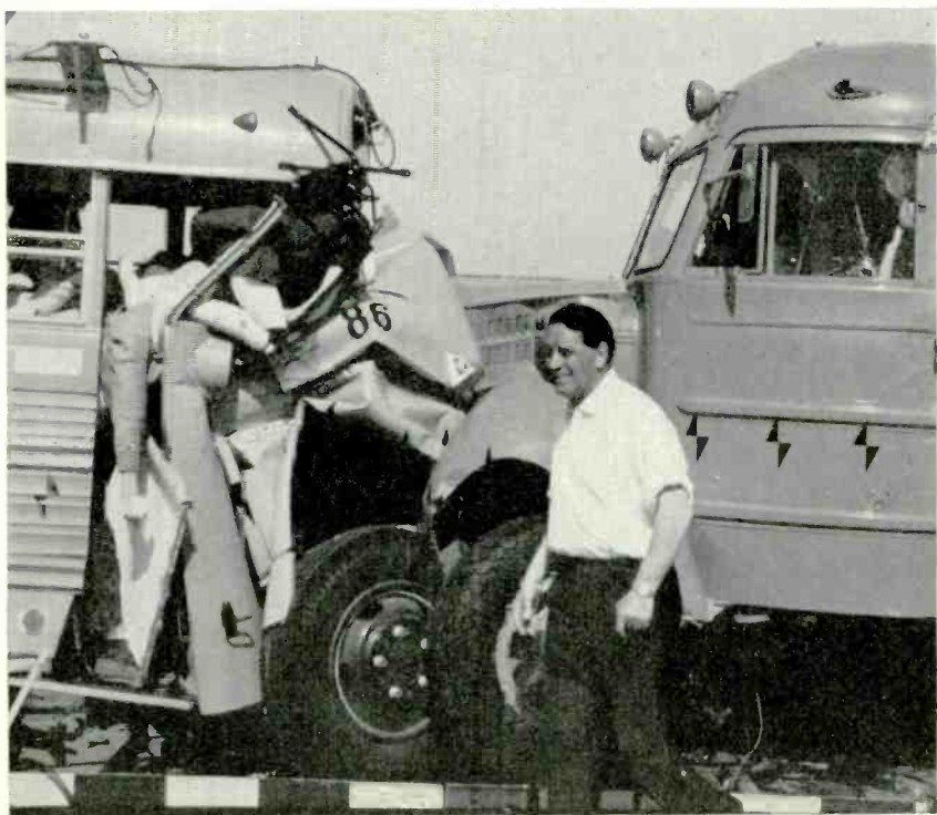
Slaughter at Speed from the television programme Examining Road Accidents . The close-up is after an experimental crash staged at the University of California between two school buses
