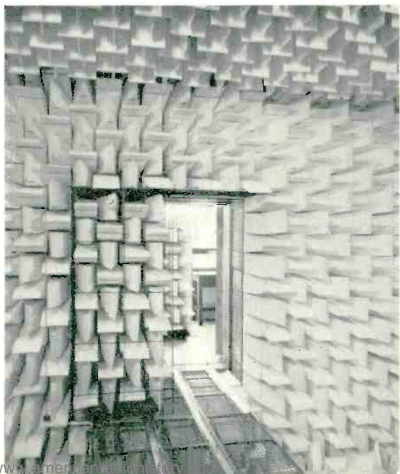
Interior of the latest of the BBC Research Department's 'dead' rooms, used for testing microphones and loudspeakers in an almost completely echo-free environment ( William R. Milligan )
