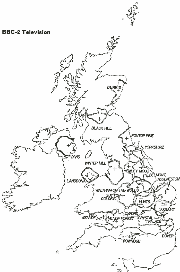
This map shows the first twenty main stations to be constructed and the approximate areas they will serve
