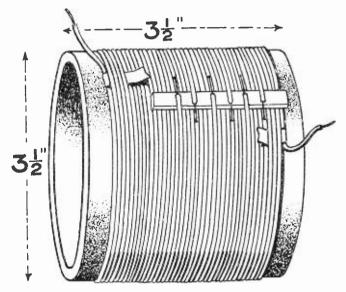
A TAPPED COIL SUITABLE FOR USE IN THE AERIAL CIRCUIT
