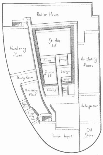
PLAN OF THE SUB-BASEMENT FLOOR, SHOWING THE STUDIOS INSIDE THE CENTRAL BRICKED-IN "TOWER"
