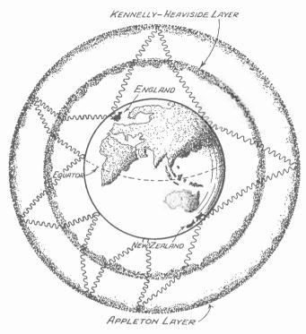
DIAGRAM OF THE PROBABLE METHOD OF SHORT-WAVE PROPAGATION, BY THE INDIRECT RAY, BETWEEN ENGLAND AND NEW ZEALAND
