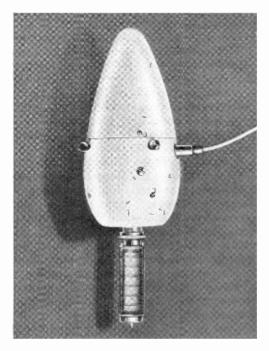
A SLACK-DIAPHRAGM CONDENSER MICROPHONE AND AMPLIFIER
