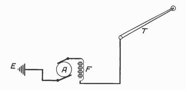
FIG. I.-MAIN CIRCUIT ARRANGEMENT OF A TRAMCAR
