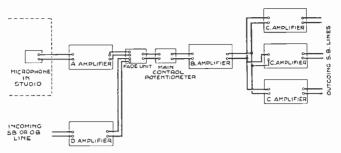
FIG. I.-TYPICAL ARRANGEMENT OF CONTROL ROOM AMPLIFIERS
