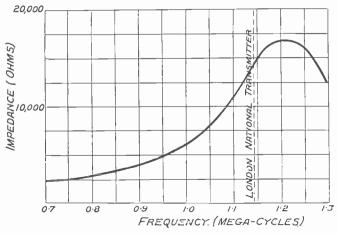
FIG. 3.—IMPEDANCE-FREQUENCY CHARACTERISTICS OF TROLLEY-BUS COPPER COIL
