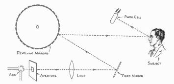
next instant, when the spot has moved to its adjoining position in the light strip, a different amount of light is reflected and the cells respond accordingly.
