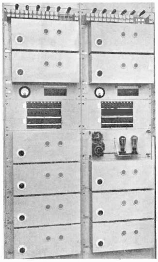
c amplifier bay with the cover removed from one amplifier  $[\ 398\ ]$
