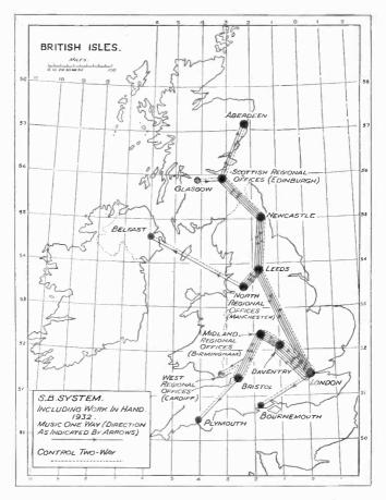
THE TELEPHONE TRUNK LINE CONNECTIONS IN THE B.B.C.'S SIMULTANEOUS BROADCASTING SYSTEM
