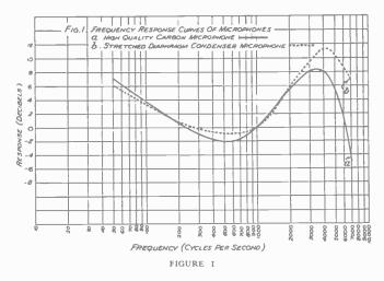
response curve of these microphones can be almost exactly equalised. A very considerable improvement in quality has been the result, and consequently Broadcasting House, in common with all Control Rooms where modern gear has been recently installed, is provided with microphone equalising circuits.
