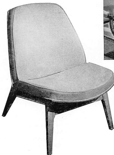
Cushioning of a new chair by H.K. Furniture is 2-in. cavity foam rubber based on 1-in. foam sheet, edged with a strip of foam rubber 1 in. thick to give a crisp finish. The whole is cemented to plywood, which is drilled for ventilation and press-studded to the frame.
